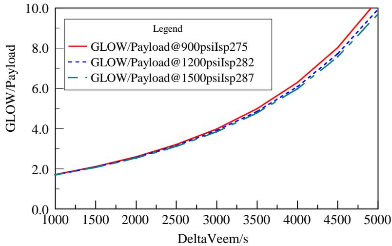
Figure 1. Ratio of GLOW to Payload for gas generator turbopump stage at pressures of 900 - 1500 psi (6 - 10 MPa).
