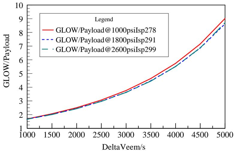
Figure 4. Ratio of GLOW to payload for pistonless pump run on liquid helium at pressures of 1000 - 2600 psi (7 - 22 MPa).
