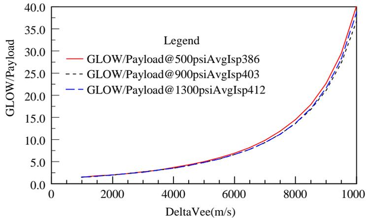
Figure 5. Ratio of GLOW to Payload for pistonless pump run on liquid helium at pressures of 500 - 1300 psi (4 - 9 MPa).
