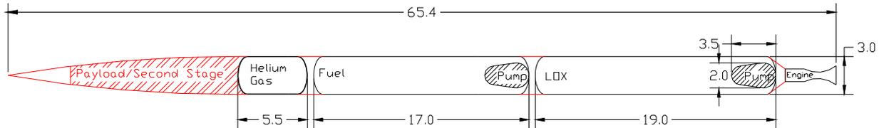
Figure 5a 25,000 lb GLOW Gas Powered Proposed Rocket Design. (Dimensions in ft.)
