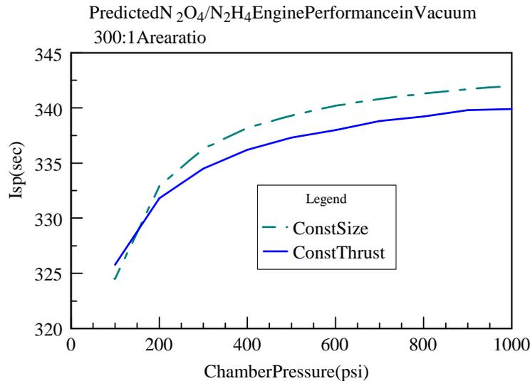
Figure 7. Aerojet engine performance as a function of pressure. Courtesy Aerojet General Corp. The engine tradeoff is normalized for either constant thrust or constant throat size.
