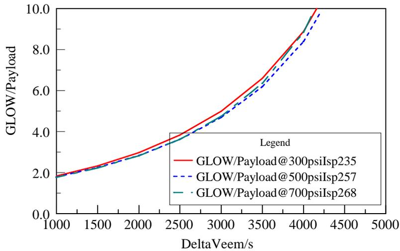
Figure 2. Ratio of GLOW to Payload for pressure-fed stage at pressures of 300, 500, 700 psi (2 - 5 MPa).
