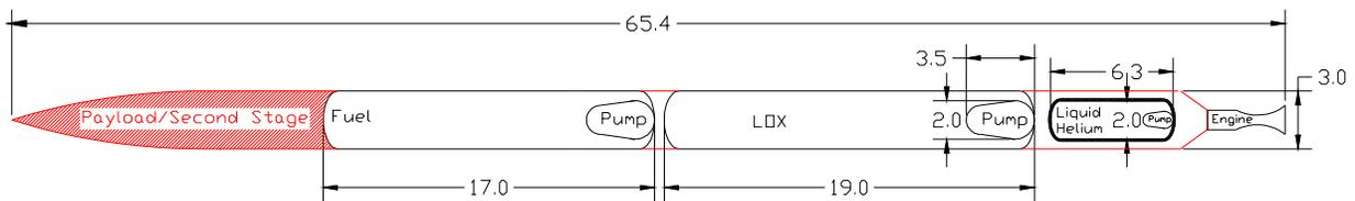
Figure 5b 25,000 lb GLOW Liquid Powered Proposed Rocket Design. (Dimensions in ft.)
