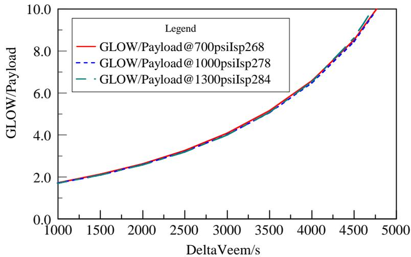
Figure 3. Ratio of GLOW to payload for gas pistonless pump at pressures of 700 - 1300 psi (5 - 9 MPa).
